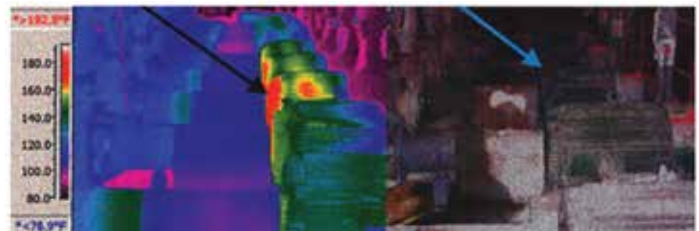
IR scans of multiple electric motors can highlight those with hot bearings indicating an imbalance or wear problem.
