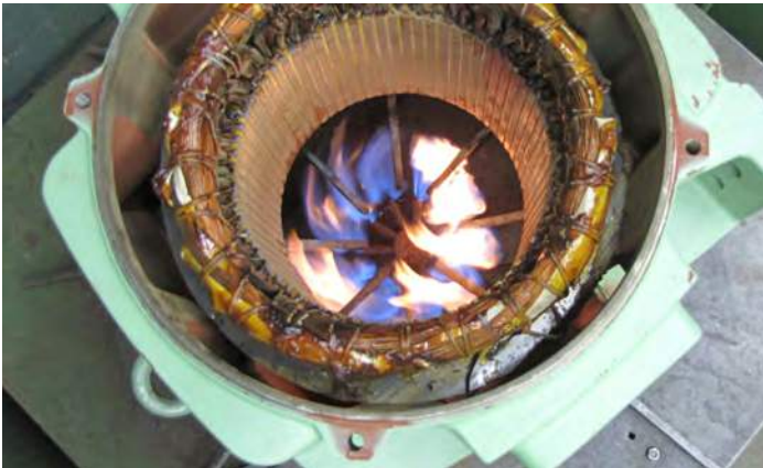
Once the winding head has been removed, the process of stripping really begins, placing a stator over a flame of roughly 400° F.
