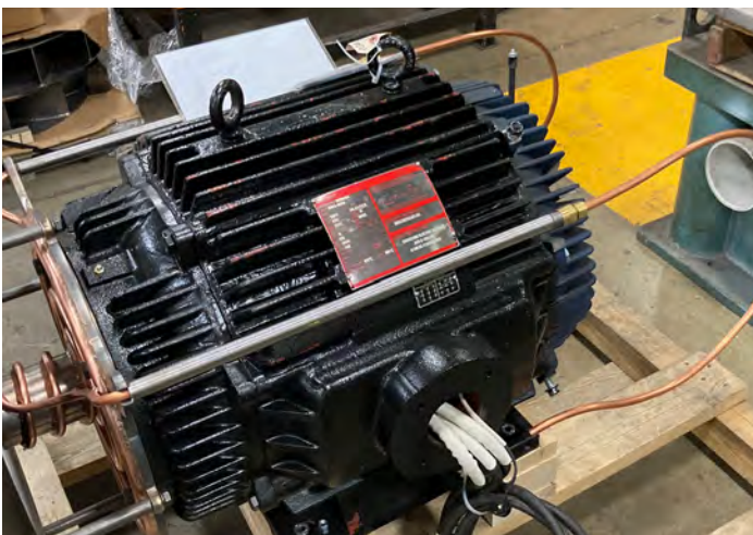
A liquid-cooled motor with hand-soldered cooling pipes — in a burnout oven, the cooling system would melt completely away.
