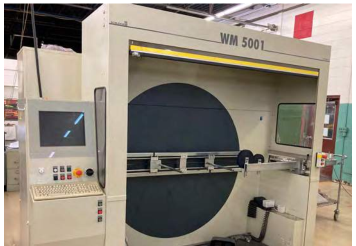
Computer-automated winding machines like this one guarantee uniform coil length for proper phase balancing.
