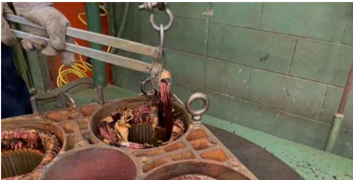
After warming, winding can be stripped out and removed manually — with much cleaner results than offered by burnout ovens.
