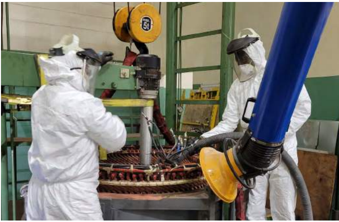
Cutting the winding head from a large engine using a circular saw.
