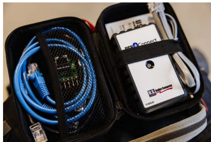
U.S. Boiler Company's new USB-Connect smartphone application requires only download of the free mobile app and the USB-Connect Bluetooth adapter kit.
