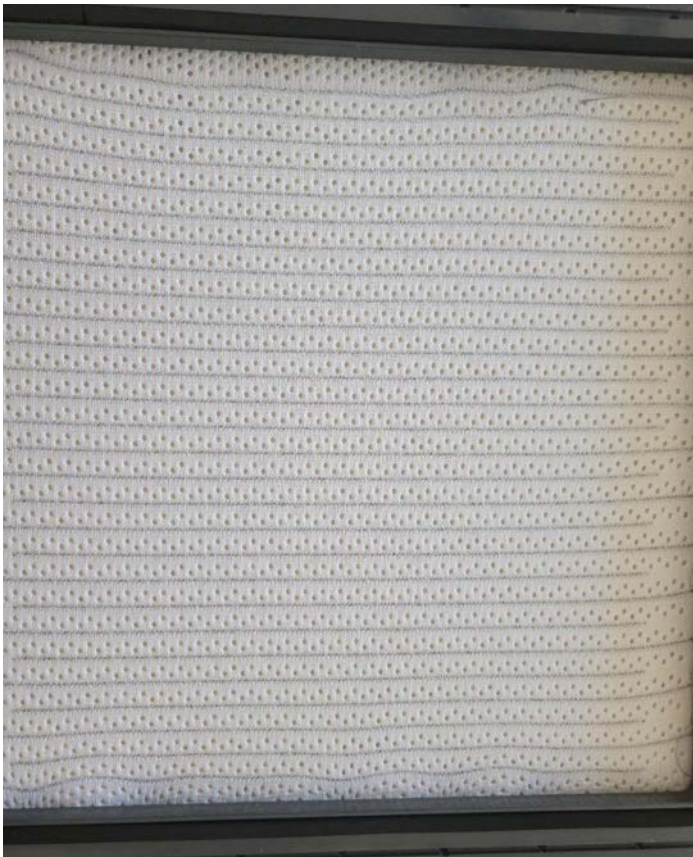
FIL-TEX is 2D textile that produces a non-thermal plasma when charged with a voltage. It catches and kills pathogens with up to 99.9-percent efficiency.
